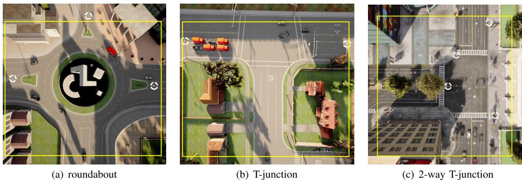
Fig. 6. Bird eye view of three driving scenarios. There are three LiDAR sensors in the roundabout scenario, two in the T-junction scenario, and four in the 2-way T-junction scenario. The white dot circle represents the LiDAR sensors, and the yellow rectangle is the detection range. The autonomous vehicle is driving from bottom to top.
